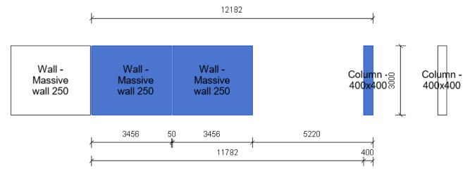
**Dimension Element** - dimension contour of one selected element by using Dimension Configuration (command below this one)
